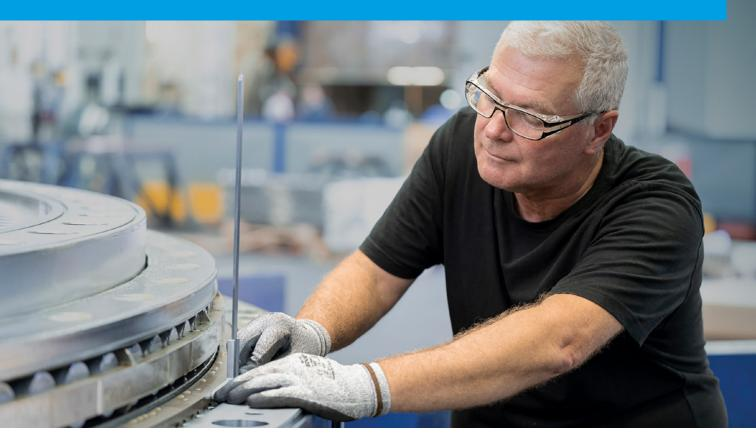
The dismounted or spare bearing is disassembled into its individual parts and checked in detail. The current condition and possibilities for further steps, such as repair, are described in our inspection report.
