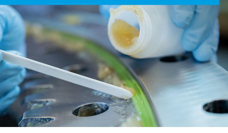
Proper relubrication is essential for the performance and longevity of your bearings. We analyze the used lubricant from the bearings to determine the current condition, and optimize if necessary.
