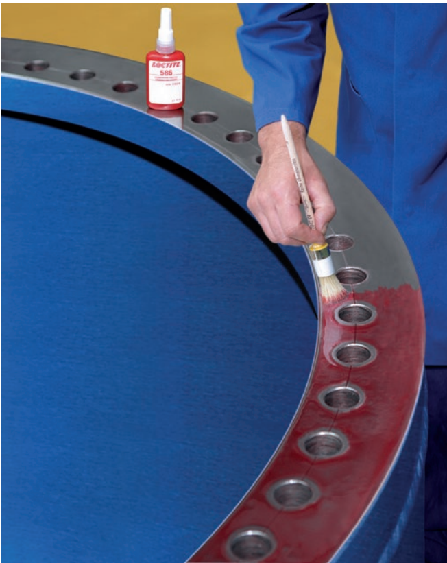
Figure 16: Application of Loctite
