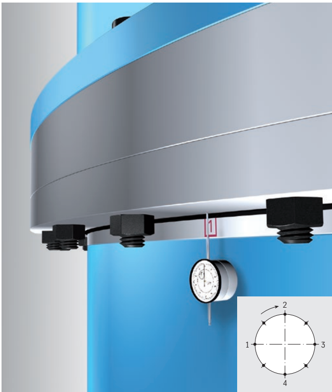
Figure 34: Basic setup for measuring the tilting clearance
