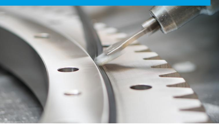
To avoid the contamination of the raceway system and uncontrolled leakage, we exchange the seals of your bearing.
