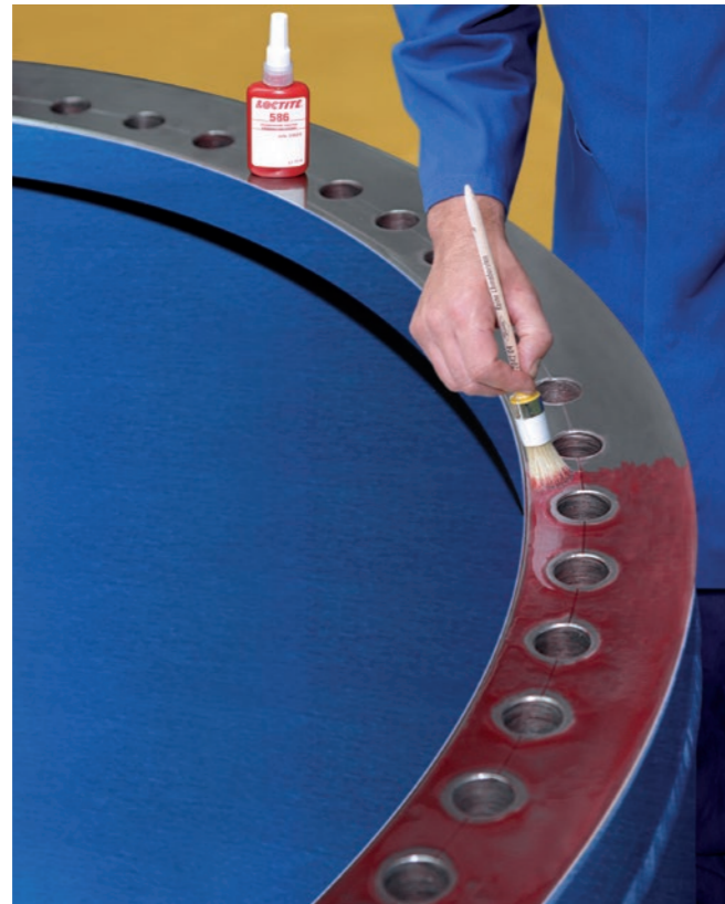
Figure 16: Application of Loctite
